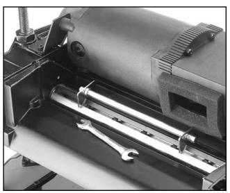
Figure 10. Knife gauge positioned on cutterhead.
